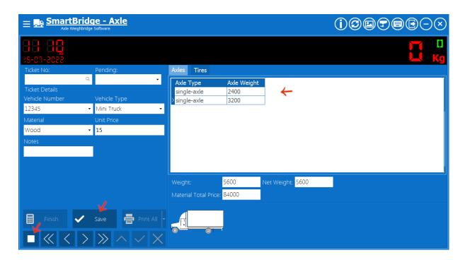
If you set the process type to "Calculating the net weight" you can add a field for the tare weight so user can fill it manually and the software will use the value in this field to calculate the net weight.
