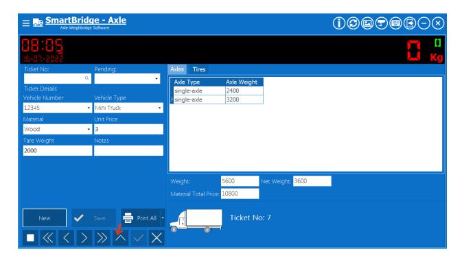
Pressing the edit button will unlock the ticket fields except the vehicle number and the vehicle type. After finishing the edit you can press the Save button to save the changes.
