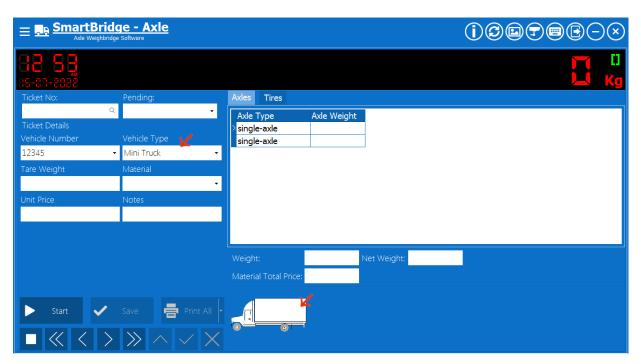
After saving the vehicle type you have to enter the axles that exist in this vehicle type, and to do so, select the vehicle type and press "Add Axle", press the button inside the axles grid to select the axle type from the list of axle types you entered
