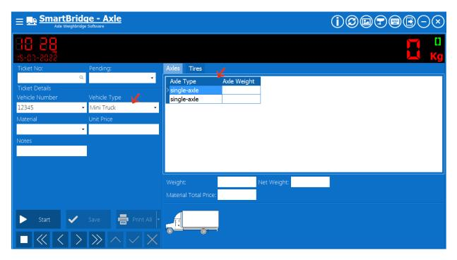
Fill all the information required in the ticket and when you are ready press the Start button and tell the vehicle driver to drive the vehicle slowly over the weighbridge. You will notice a flashing warning symbol on the black screen next to
