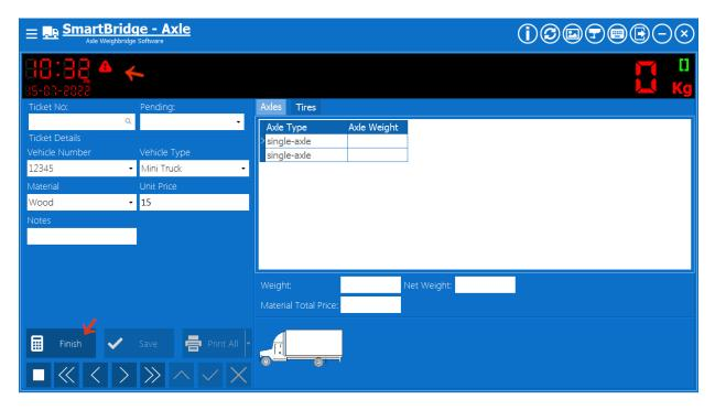
After pressing the Finish button the software will show the axles weight. You can save the ticket by pressing the Save button. To cancel the ticket you can press the cancel/stop button and nothing will be saved.
