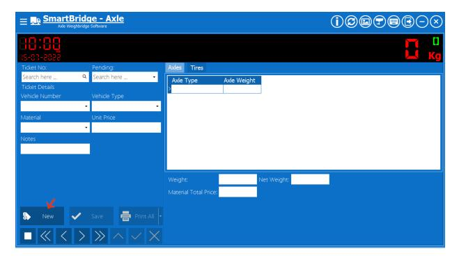
Fill the vehicle plate number and the vehicle type, after selecting the vehicle type the software will show the axles that exist in this type.
