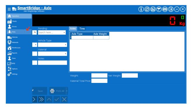
This screen has two tabs, In the Axle Types tab you can enter the types of axles that you want to work with. If you set the Process type to "Calculating overweight fine" as we described before, then also you should enter the max allowed weight of each axle type, the software will calculate the fine when the axle weight exceeds the max allowed weight of the axle using the fine slices as we will see later.
