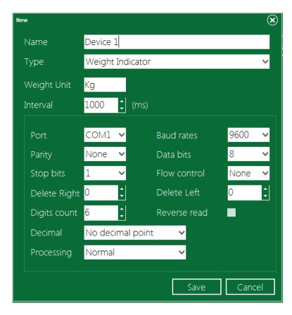
Select the port that connected to the indicator and set its properties (Baud rates, Parity, Data bits...) to make it compatible with the connected indicator. Usually you can find the suitable port settings in the indicator manuals.
