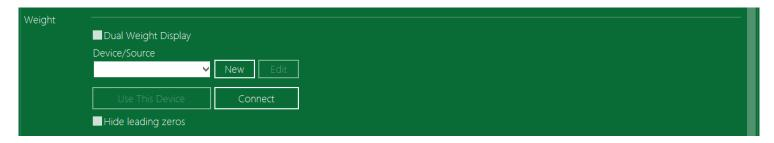
To add a new weighing device/source, press "New" button, this will show the New device window. SmartBridge professional can receive the weight value from three different sources/types:
