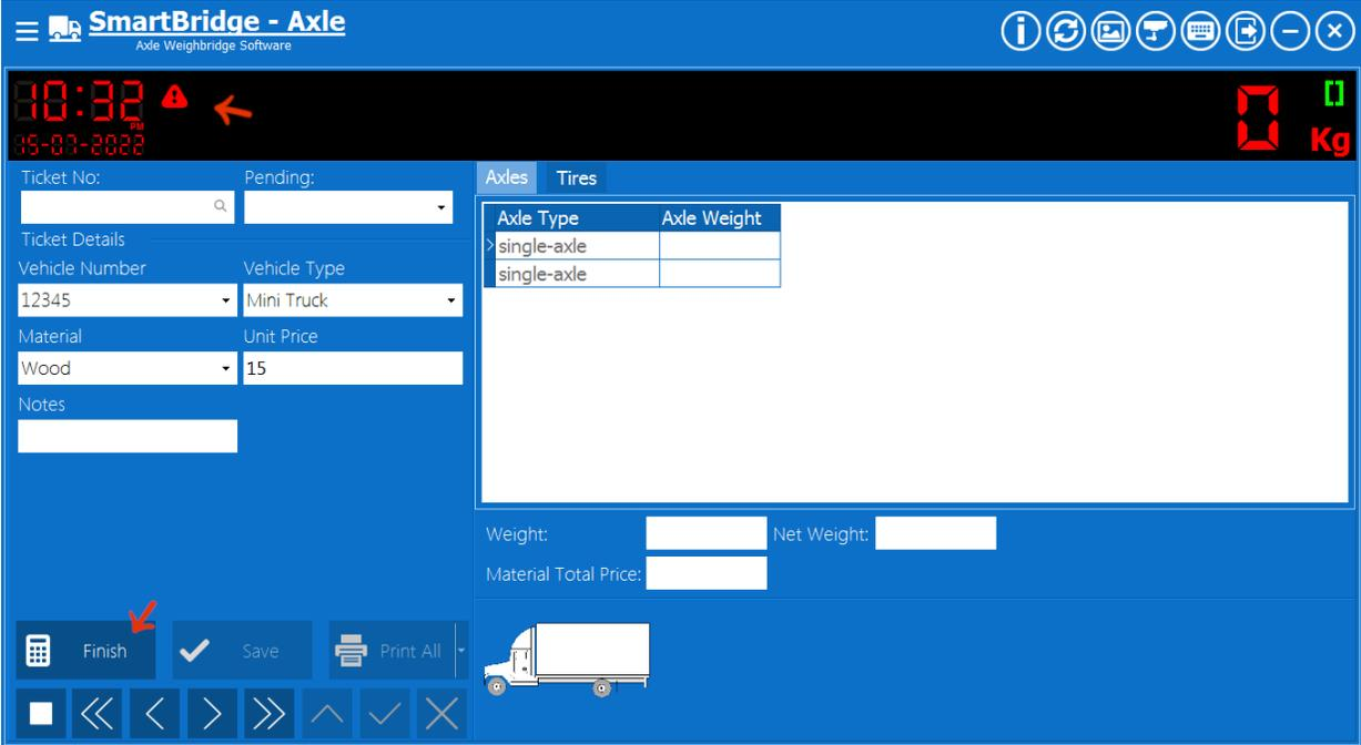
After pressing the Finish button the software will show the axles weight. You can save the ticket by pressing the Save button. To cancel the ticket you can press the
