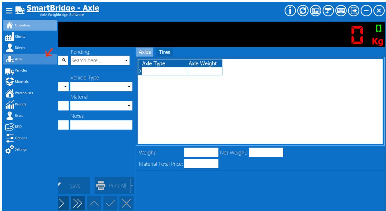
This screen has two tabs, In the Axle Types tab you can enter the types of axles that you want to work with. If you set the Process type to “Calculating overweight fine” as we described before, then also you should enter the max allowed weight of each axle type, the software will calculate the fine when the axle weight exceeds the max allowed weight of the axle using the fine slices as we will see later.
