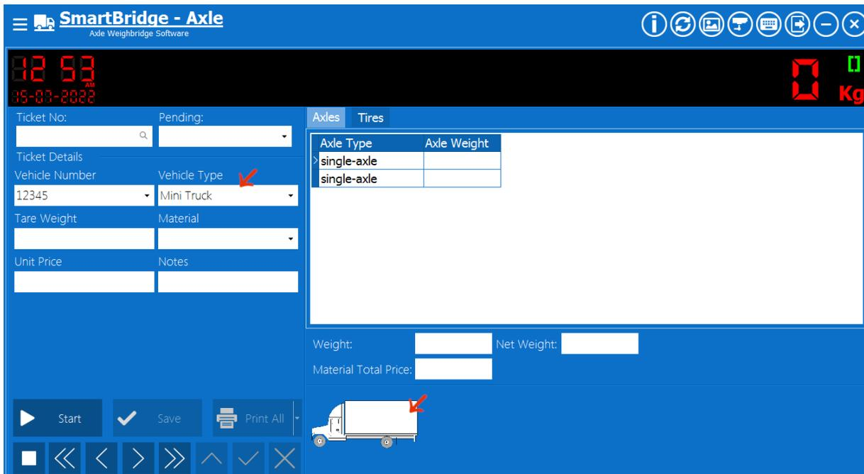
After saving the vehicle type you have to enter the axles that exist in this vehicle type, and to do so, select the vehicle type and press "Add Axle", press the button inside the axles grid to select the axle type from the list of axle types you entered
