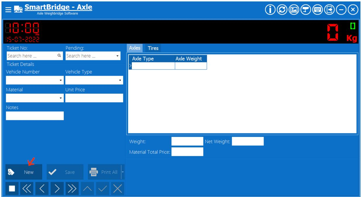
Fill the vehicle plate number and the vehicle type, after selecting the vehicle type the software will show the axles that exist in this type.
