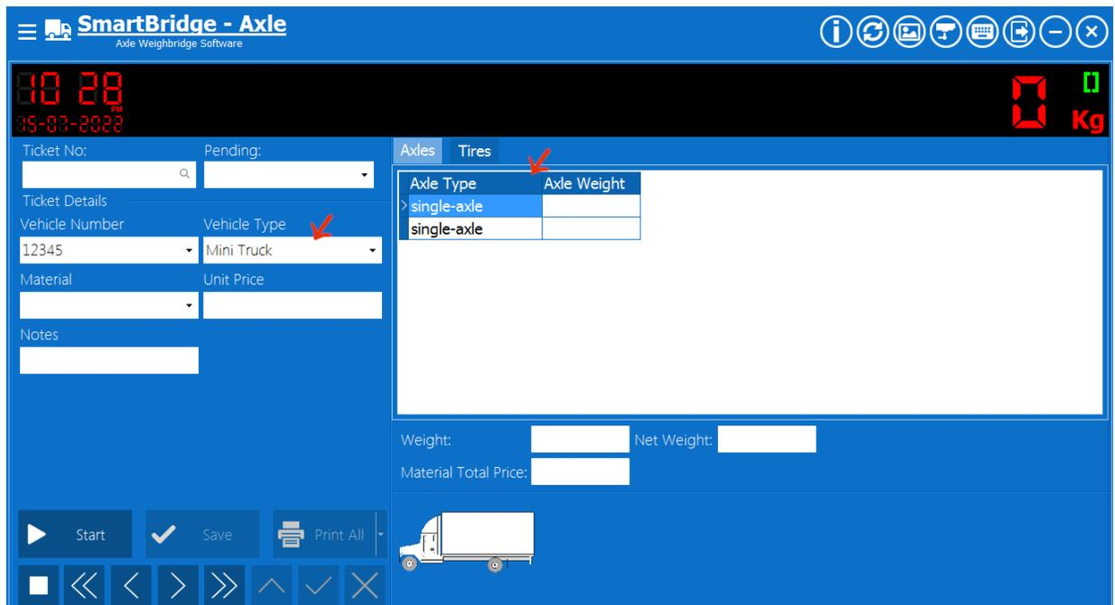
Fill all the information required in the ticket and when you are ready press the Start button and tell the vehicle driver to drive the vehicle slowly over the weighbridge. You will notice a flashing warning symbol on the black screen next to
